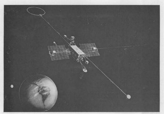
OGO IN ACTION. This artist's conception illustrates the in-orbit positions of OGO's geophysical experiments. Paddles of solar cells to right and left of main body of spacecraft provide 28-volt DC nominal power supply for the satellite. Long and short booms carry antennas, and experiments which must be isolated from main body of the spacecraft.
